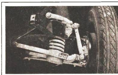
INDIVIDUAL SPRINGING on the Plymouth is shown above. It is simple, accessible, dependable. A double-acting shock-absorber is a part of each wheel suspension.
